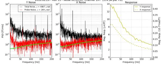
Notice the significant difference between the technical Y noise. The digitization was much more noticeable with the 250 Hz filter – the two must be related.
