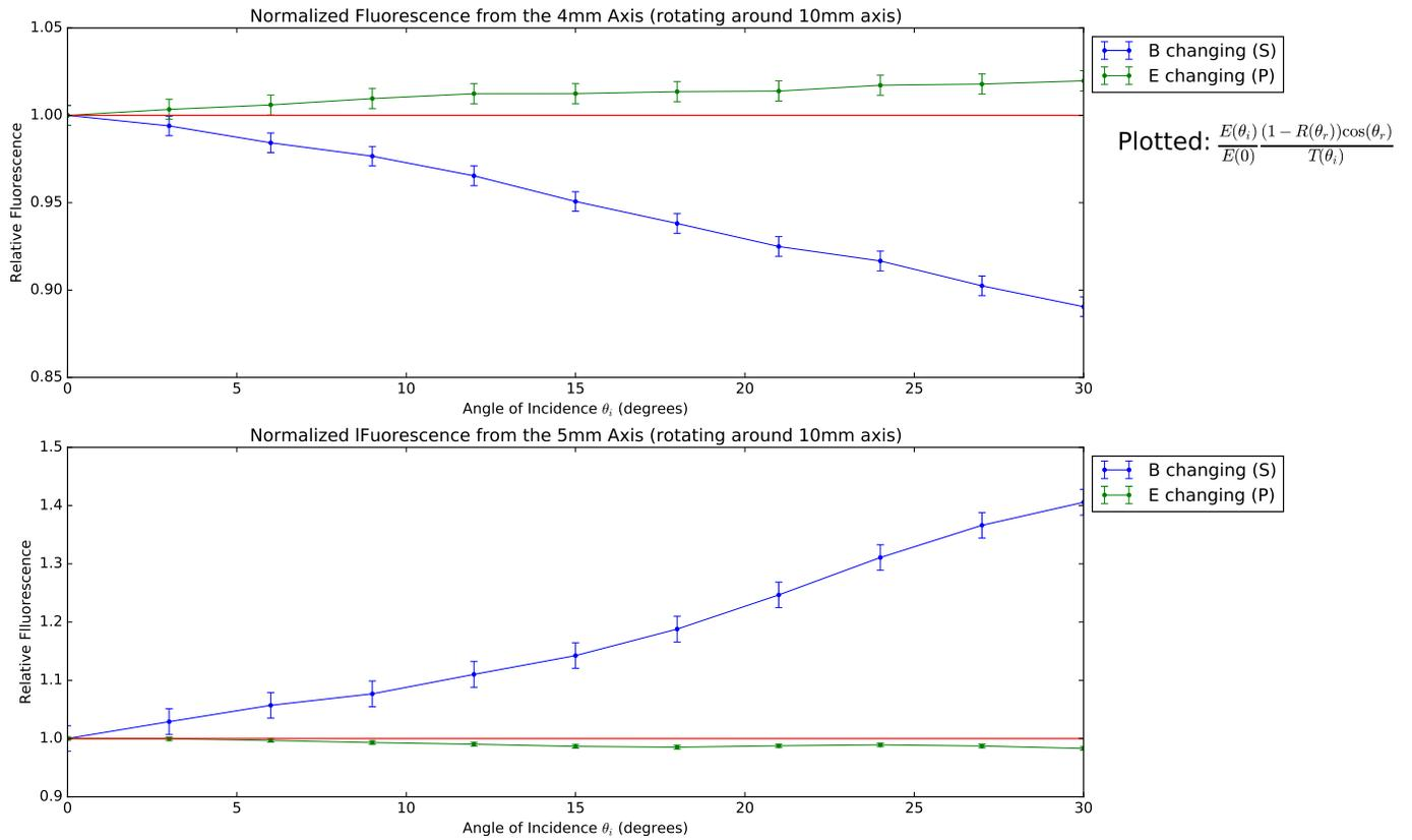
Figure 2: Fluorescence while rotating around the 10 mm axis. In the top plot the beam is propagating along the 4mm axis. In the bottom plot the beam is propagating along the 5 mm axis. These plots clearly show that the fluorescence responds to the orientation of the magnetic field and not the electric field.
