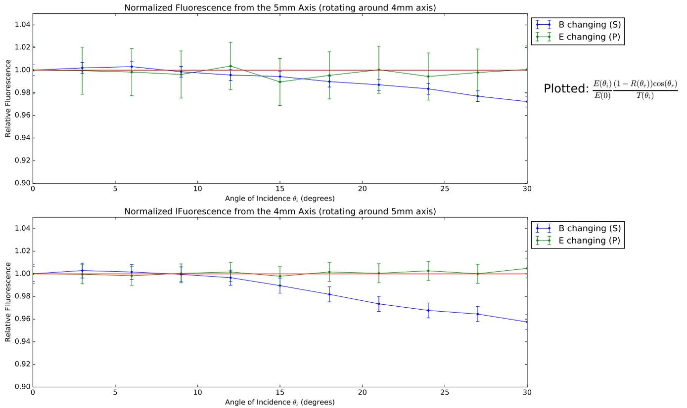
Figure 3: The top plot shows propagation along the 5mm axis and rotation around the 4 mm axis. The bottom plot shows propagation along the 4 mm axis and rotation around the 5 mm axis. These plots also clearly show the dependence on the magnetic field.
