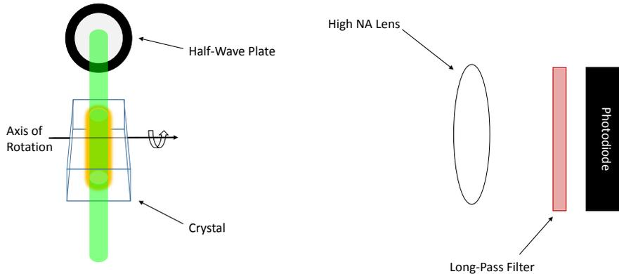
Figure 1: The Experimental setup. The crystal is mounted in a Gimbal mount with an axis of rotation parallel to the page. The Laser beam is coming roughly out of the page. The filter we used was a red transmission filter with a cutoff low enough to transmit the fluorescence. The photodiode was a Thorlabs PDA36A (CHECK THIS).
