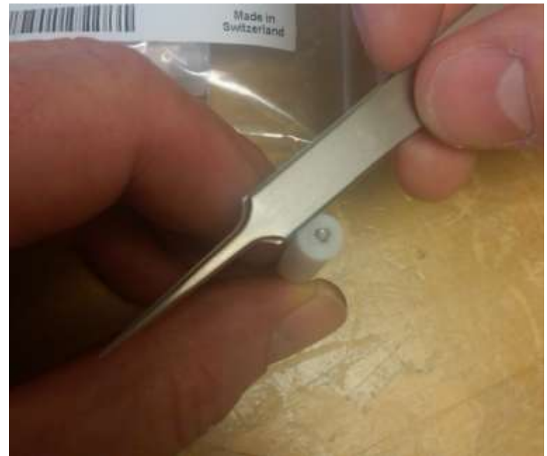
Ignition aid mounted on insertion tool ready to be installed on anode
