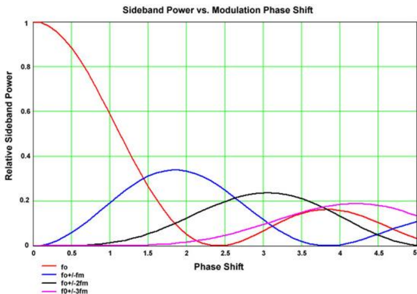
Figure 2 Sideband Power Versus Phase Shift
