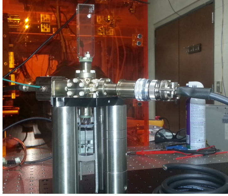
Figure 8.2: Image of the double vacuum system. The 2D-MOT chamber with dispenser is on top. The 3D-MOT science region is below in a ColdQuanta hexagonal vacuum cell. The dispenser electrical connection can be seen on the right and the ion pump is in the back left.
