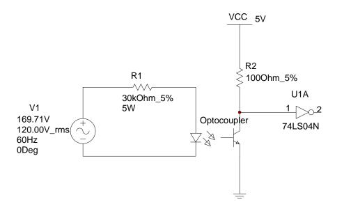
The optocoupler is part number 6n137. The output of the not gate goes to the FPGA to trigger. A 100 nF capacitor goes between pins 1 and 8 of the optocoupler.
