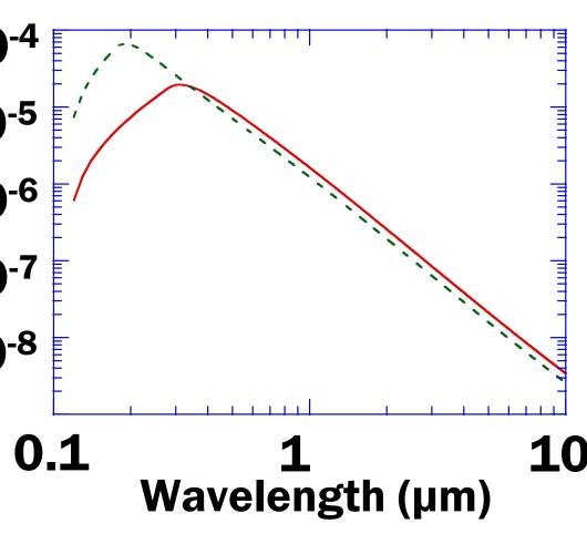
**Theoretical conversion** efficiencies of mixing to sideband beam powers for different pressures of  $H_2$ ; the solid red is 0.33 atm, and the dashed green is 0.08 atm. We expect that the conversion efficiency curve for the current **10** experiments with  $D_2$  will be qualitatively similar.
