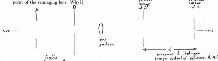
Calculate the etendue U for the external images as drawn above. (The value of U should agree with the etendue determined from the internal measurements because the etendue is not changed by a lens that is large enough to accommodate all the rays exiting the instrument.)
