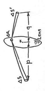
Figure 3/1-2. Concept of conservation of etendue, U. The magnification of elements of object area As is neatly compensated by distances p,q, leaving the element of solid angle and hence the element of etendue unchanged by the lens action.
