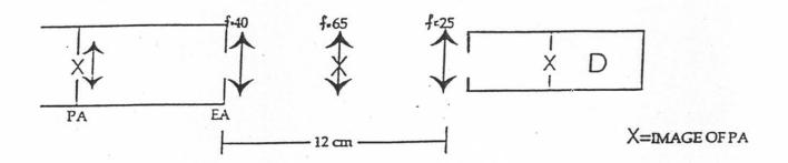
In this diagram, the "instrument" is on the left and the detector is on the right. In this diagram "X" marks either the PA aperture or its images.
