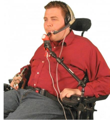
Figure 5: An ALS patient in a sip-and-puff controlled wheelchair
